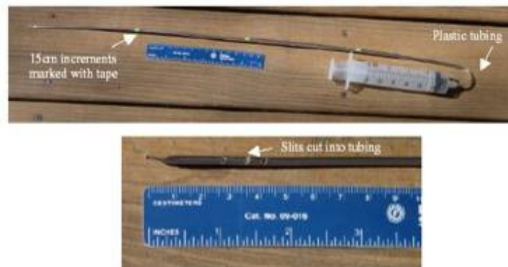
Figure 10 Photograph of a soil probe (sipper) used to take interstitial pore water samples to measure pore water salinity (Roman et al. 2001).
