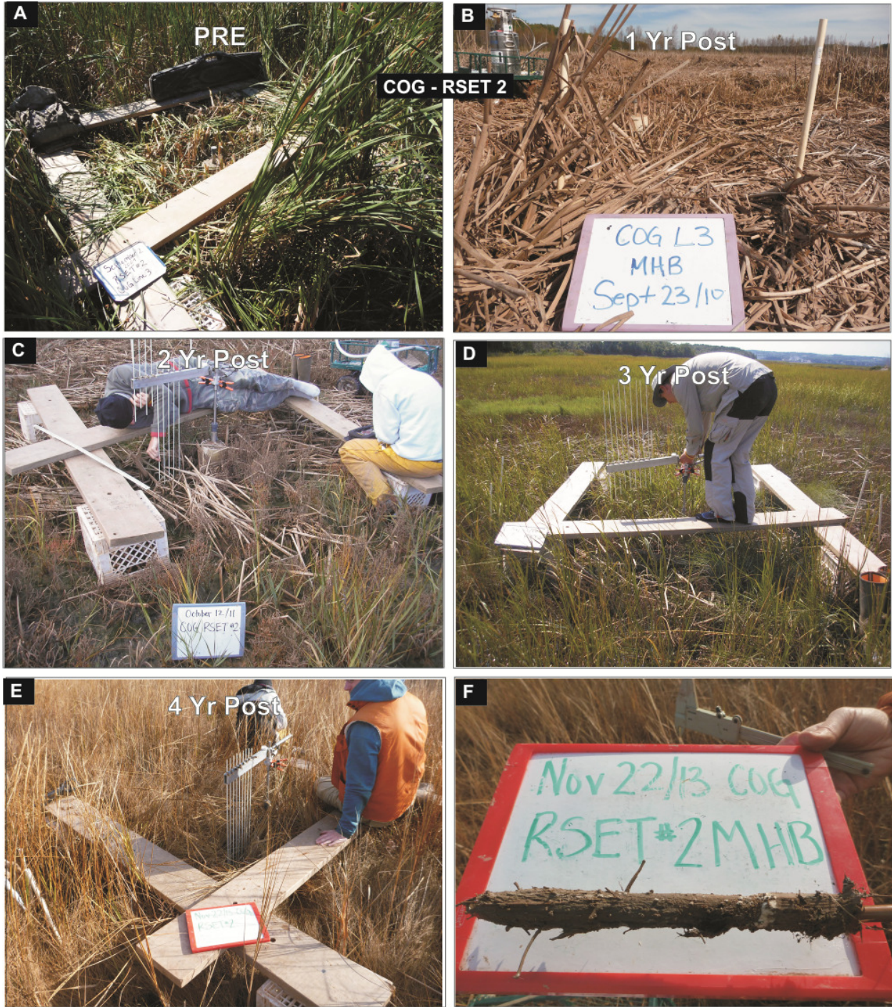
Figure 25 RSET-02 at COG a) Pre (19 August 2009), b) Year 1 Post (23 September 2010), c) Year 2 Post (12 October 2011), d) Year 3 post (20 August 2012) and e) Year 4 post (22 November 2013). Photo (f) shows an example of a marker horizon core. Photographs taken by CBWES Inc..
