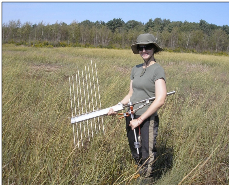
Figure 12 The nine measure pins of the RSET. Photograph by CBWES Inc.
