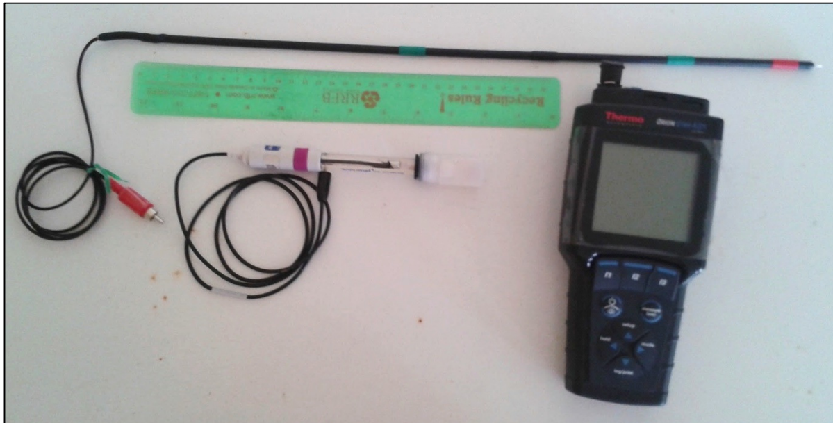
Figure 15 Constructed platinum electrodes (top), accumet calomel reference electrode (bottom) and Thermo Scientific Orion Star A221 Milivolt Meter (Photo: C. Skinner 2013).
