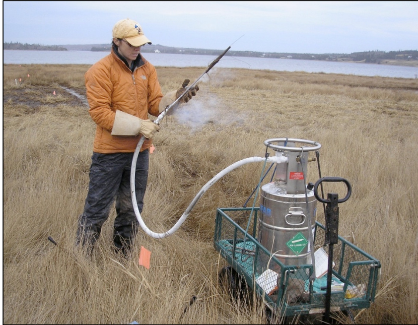
Figure 13 Marker horizon sampling with the cryogenic corer (with stainless steel tubing and copper “bullet”) at Lawrencetown Lake Reference Site. Photograph taken by B. Lemieux, December 2011.
