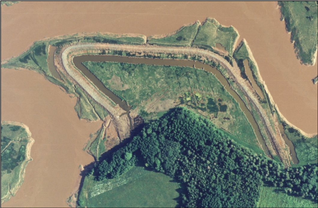
Figure 3 COG following the construction of the dyke and conversion to freshwater impoundment. 1992 aerial photograph.
